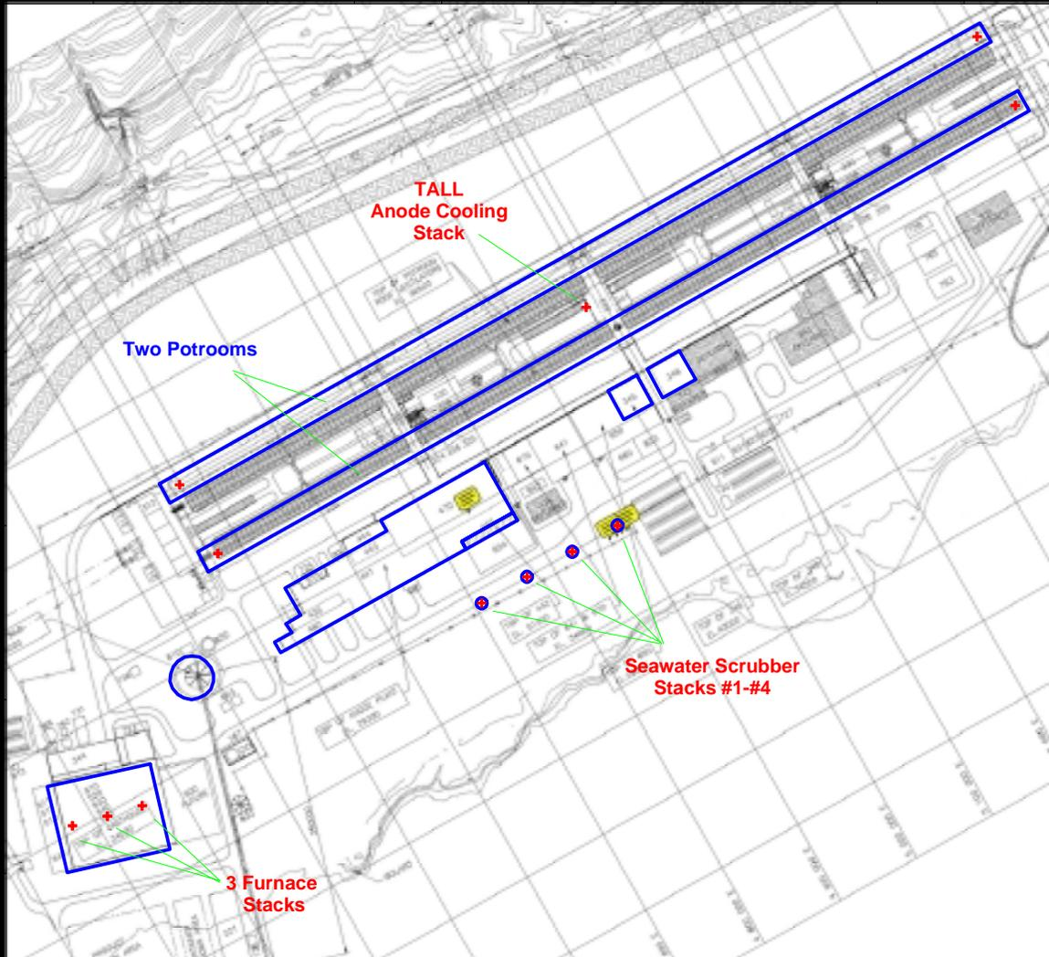
Figure 2-1. Plan of the Alcoa facility showing building locations and the emission sources. Note that the location of the potrooms was extracted from a separate more detailed map.
